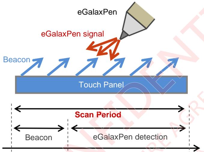
The period of eGalaxPen detection is divided into slices. The signal received can be presented on the time slices and compose an image called Pen Data, as shown below.
