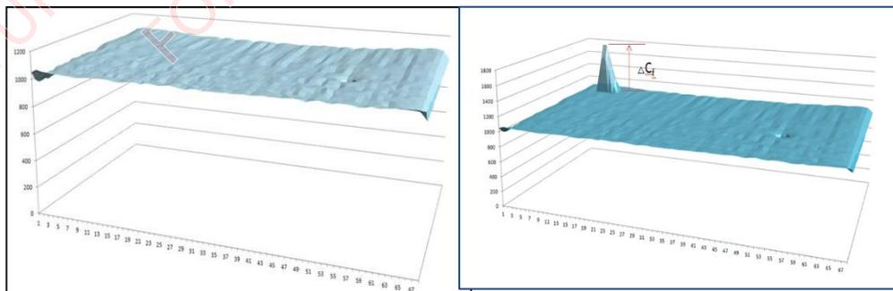
Calculating the change from baseline to the current Raw Signal, we can derive L1 signal, which represents the touch signal.
