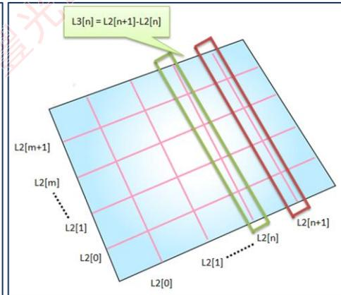
$Touch\% = \Delta C_f / C_f$ , which represents the ratio of the signal changed by a finger touch to the signal received from the Rx electrode without a touch. This value is subject to the touch screen design and the system mechanism.
