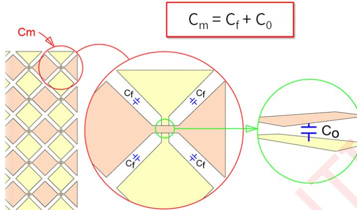
$C_f$  = fringe capacitance, which can be changed by a finger touch ( $\Delta C_f$ ).
